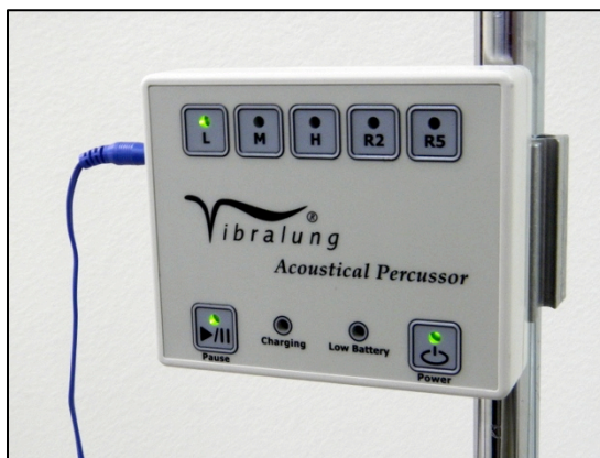
Vibralong Acoustical Percussor Treatment Control Unit (TCU) mounted with the supplied pole-mount slide bracket and optional pole-mount clamp.
