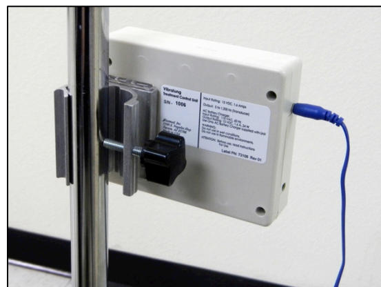
Vibralong Acoustical Percussor Treatment Control Unit (TCU) mounted with the supplied pole-mount slide bracket and optional pole-mount clamp.
